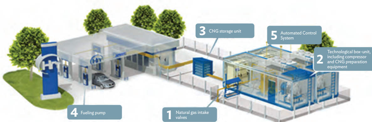
Figure 17: Working Design of a Compressed Natural Gas Fueling Station with Refueling Capacity of 2100 Cubic Meters per Hour
