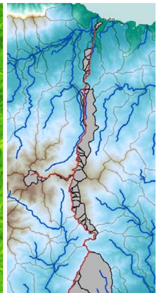
Left: detail of the NEXTmap Digital Elevation Model (DEM) for Timor-Leste, overlaid with the derived catchments and river network. Middle: slope map derived from the DEM. Right: the derived hydrological catchments (light brown outlines), the river network (blue lines) and the road catchments (grey areas with black outlines) over a backdrop of the DEM. NEXTmap © InterMap/BlackBridge SARL.
