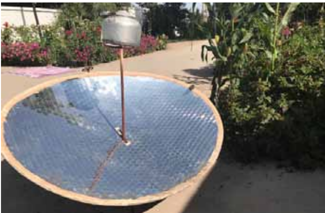
A typical parabolic solar cooker, one among the 98,000 distributed to low-income households across three counties in the PRC. Photo credit: Beijing Harmonious Energy Development.
