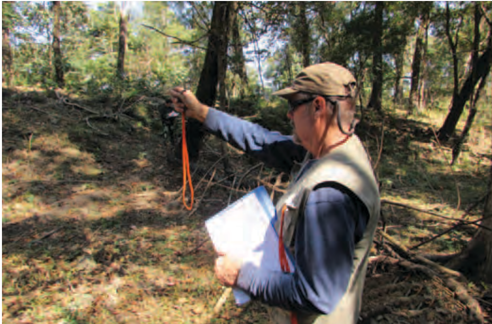
“Plotless” overstory tree sampling. This approach involves the use of wedge prism to survey trees based on distribution and size in a site (photo by ADB).
