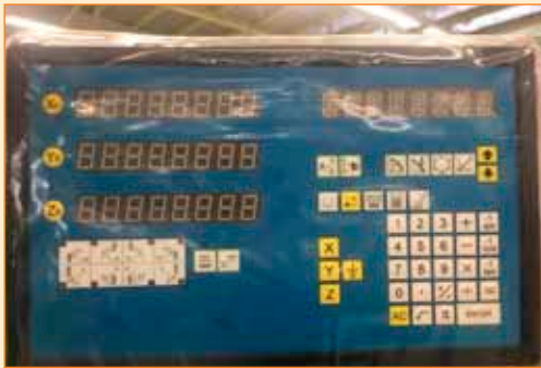
■ Conventional digital readout. Close-up photo of a conventional digital readout.
