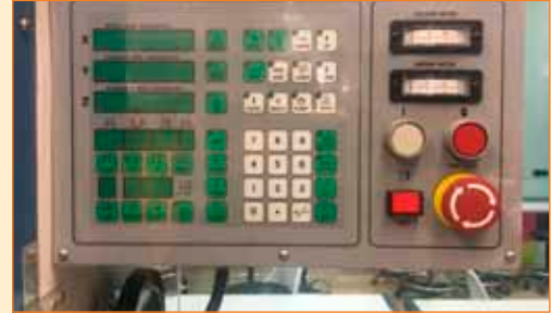
■ Digital readout. A digital readout in a conventional surface grinder.
