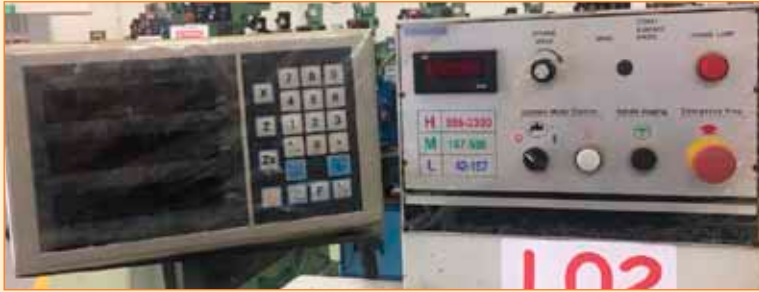
■ Digital readout. A digital readout in a conventional turning (lathe) machine.
