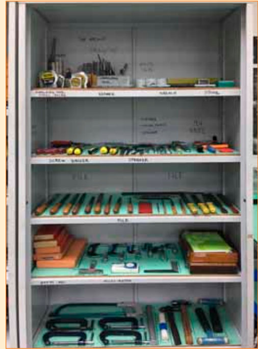
■ Tooling cabinet. Proper labeling and arrangement of tools in a tooling cabinet.
