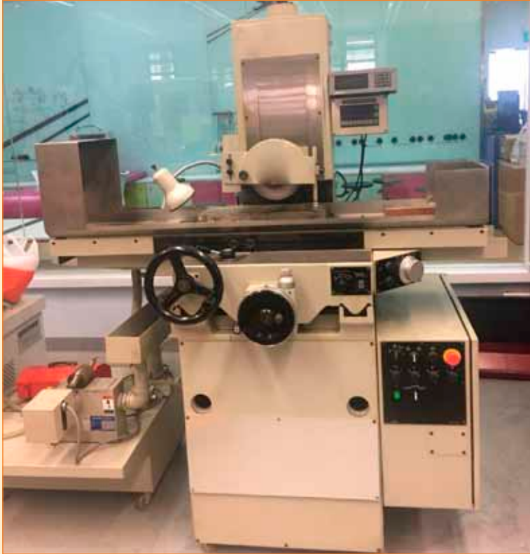
■ Conventional surface grinding machine. A conventional surface grinding machine with digital readout.
