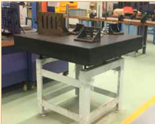
■ Granite table. Close-up photo of a granite table in a measuring station.
