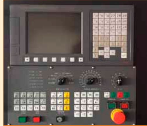
■ CNC controller. Close-up photo of a CNC turning (lathe) controller.
