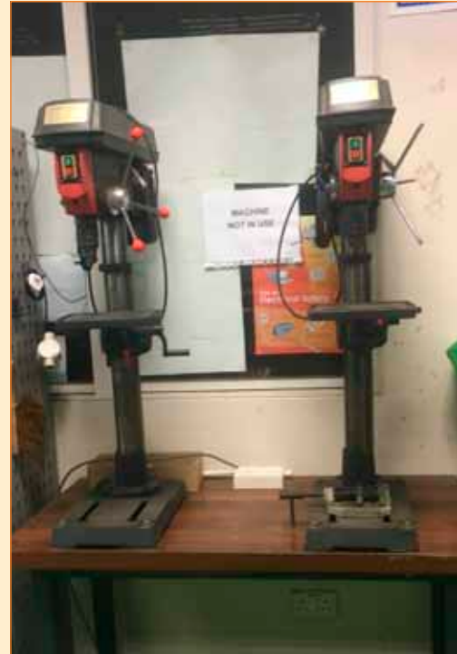
■ Drilling machine. A drilling machine in a conventional turning (lathe) machine workshop.
