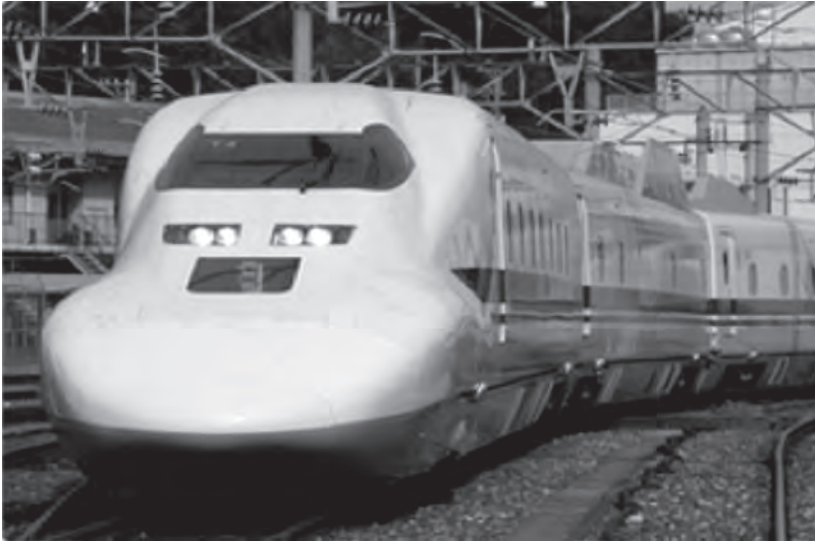
Doctor Yellow. This shinkansen electrical and track inspection train runs regularly to detect needed repairs (photo by Central Japan Railway Company).
