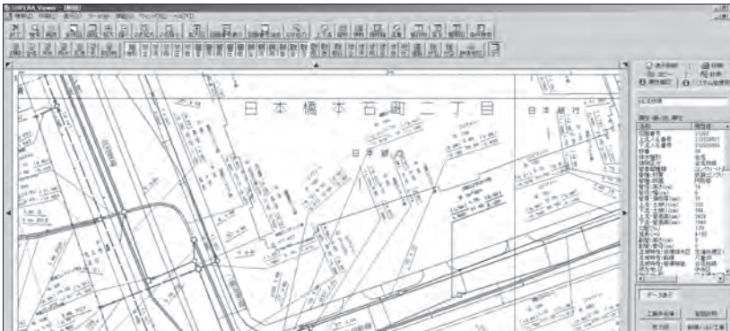
Figure 6.2: Ledger Information System of Tokyo Metropolitan Government Bureau of Sewerage (Example of a Screen)
