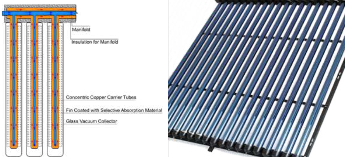
Figure 7: Direct-Flow Tube Collector with Vacuum-Insulated Glass Tubing
