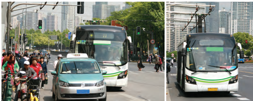
Opportunity charge system for battery electric buses in Shanghai, People's Republic of China. Source: Asian Development Bank.
