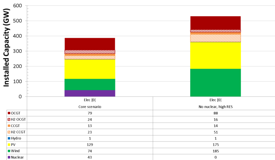
Figure E. 8 Comparison of the generation portfolio for Electric pathway with and without nuclear technology
