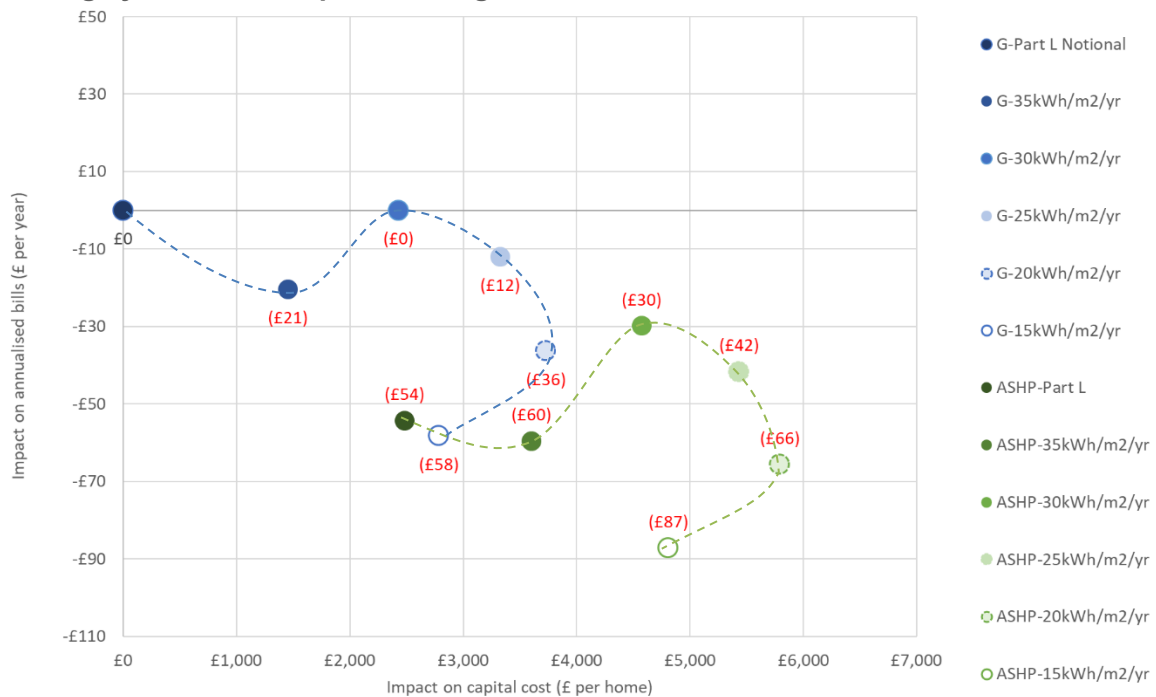
Figure 5.10 Relative running and capital costs for a semi-detached house with different heating systems 77 and space heating demand in 2020
