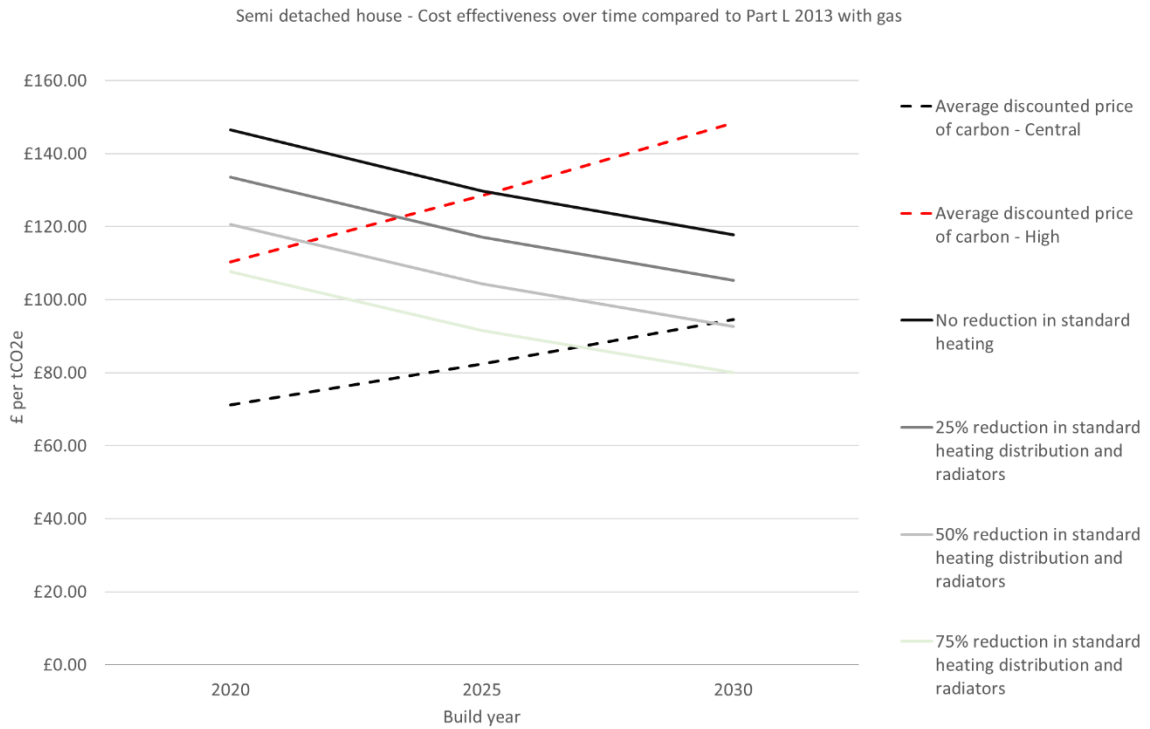
Figure G.6 Varying the scale of the reduction in heating distribution costs for ASHP-15kWh/m 2 /yr specification
